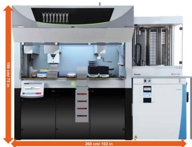
Figure 1: The Fluent assay workstation. A Fluor 780 is shown, equipped with an eight-channel Flexible Channel Arm, a Multiple Channel Arm 384 and a Robotic Gripper Arm. A Carousel is integrated onto the right hand side of the instrument, along with the latest generation of CO 2 incubator. An Infinite® M1000 PRO microplate reader is located below the Dynamic Deck. The dimensions of the compact system are indicated.
