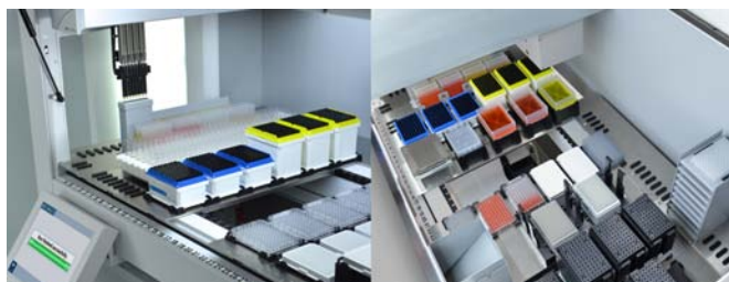
Figure 2: Dynamic Deck with six ANS/SLAS positions in the depth, equipped with six boxes for disposable tips for the Flexible Channel Arm on the left. Blue colour code for 200µl and yellow colour code for 1000µl disposable tips. Top view of the Dynamic Deck on the right showing nested disposable tips, positions for troughs, active carrier for the Multiple Channel Arm 384 and a hotel in the back.
