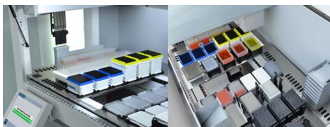
Figure 2: The Dynamic Deck can accommodate ANSI/SLAS-format carriers six deep on the worktable. (Left) Instrument equipped with six boxes of disposable tips for the Flexible Channel Arm (blue = 200 \mu l, yellow = 1,000 \mu l). (Right) Top view of the Dynamic Deck showing positions for nested disposable tips, troughs, the active carrier for the MCA 384 and a hotel at the rear.
