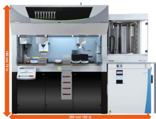
Figure 1: The Fluent cell-based assay workstation. A Fluent 780 is shown, equipped with an eight-channel Flexible Channel Arm, a Multiple Channel Arm 384 and a Robotic Gripper Arm. A Carousel is integrated onto the right hand side of the instrument, along with the latest generation of CO 2 incubator. An Infinite M1000 PRO microplate reader is located below the Dynamic Deck. The dimensions of the compact system are indicated.
