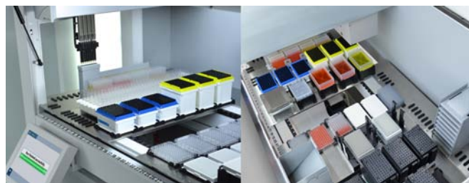
Figure 2: Dynamic Deck with six ANSI/SLAS positions in the depth, equipped with six boxes for disposable tips for the Flexible Channel Arm on the left. Blue colour code for 200µl and yellow colour code for 1000µl disposable tips. Top view of the Dynamic Deck on the right showing nested disposable tips, positions for troughs, active carrier for the Multiple Channel Arm 384 and a hotel in the back.
